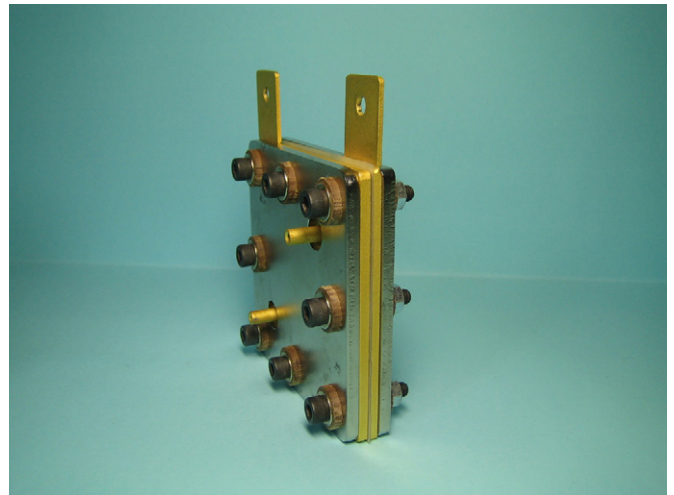
Fig. 7. Prototype one-cell PEM fuel cell stacks with gold-plated titanium bipolar plates.
